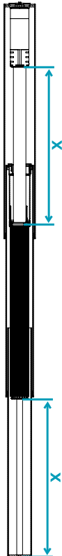
Fig. 3: Synchronous movement of the Middle Tube results in the distances marked by x remaining equal. This is not affected by the height of the Table Top.
