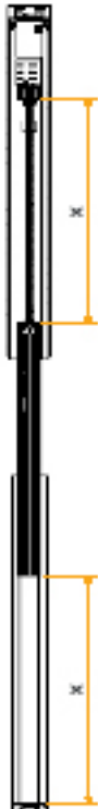
Fig. 4: Synchronous movement of the middle tube results in the distances x being the same at all times independently from the current height (middle tube removed for easier demonstration).
